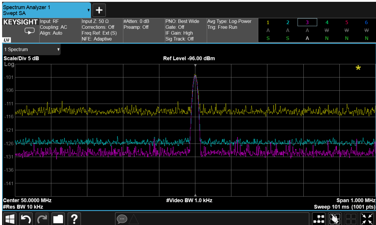
Figure 8. In these signal measurements, DANL becomes progressively lower after reducing resolution bandwidth (yellow), reducing input attenuation (blue), and switching to log power averaging (purple).
