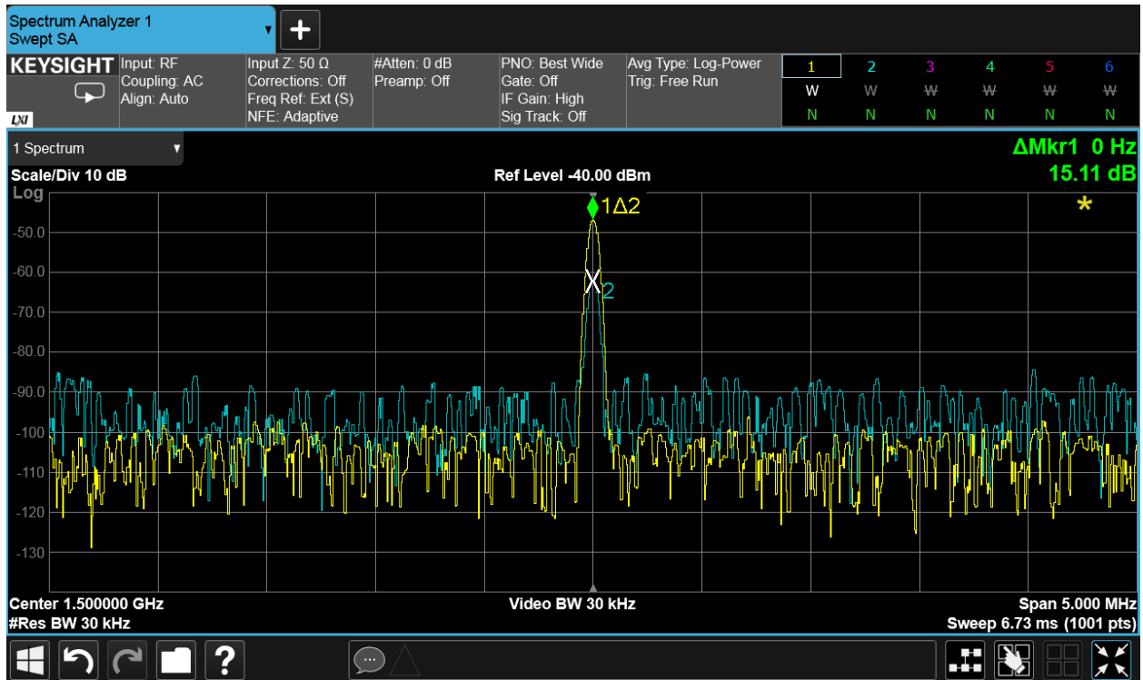
Figure 16. Because the signal analyzer accounts for input attenuation and reference level, a difference in the apparent second-harmonic amplitude is due to distortion from the analyzer.
